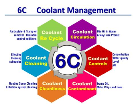
The 6C, as a concept is presented here is to demonstrate how to institutionalize a coolant management system that will effectively increase coolant life to its designed life expectancy levels thereby reducing consumption, and improving performance of the machine tool in terms of tool life, component finish, machine down time, and finally reducing disposal costs.
