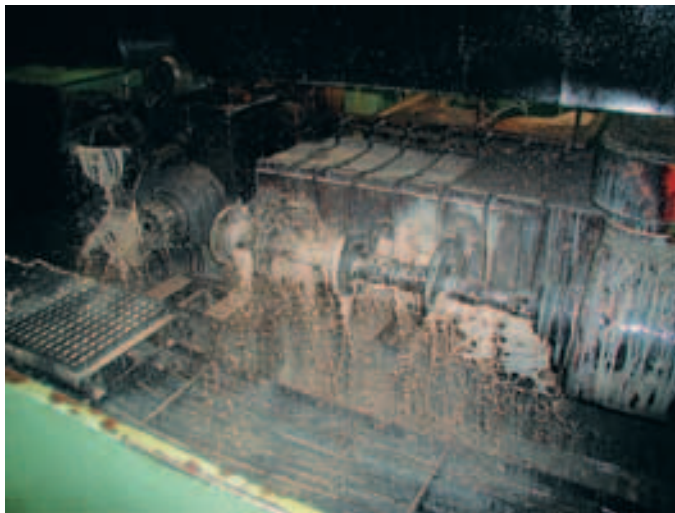
Blasocut Kombi 883 on the job. This is only one of the production line stations – here without workpiece – showing just how much cutting fluid is required overall for crankcase machining.
