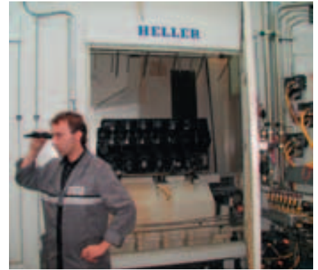
Maintenance foreman Heiko Klein never has any cutting fluid problems. He just checks the emulsion once daily on the machine and once weekly in the laboratory.
