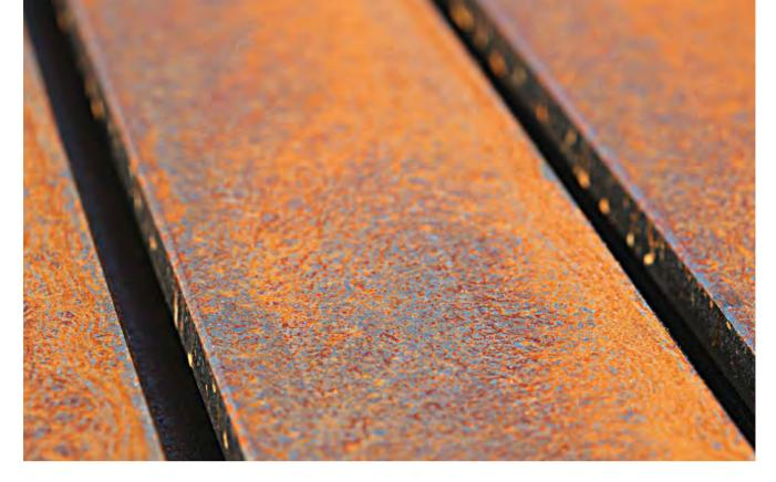
tests show that corrosion becomes increasingly likely when chlorides are above 300 ppm.
