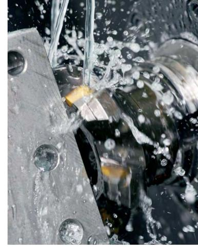
When concentration levels are low, the components in the fluid that provide corrosion protection are insufficient to protect the metal surfaces. For most metalworking fluids, low concentrations are those generally below 4%. If concentration is lean, simply add sufficient concentrate to bring the system within the recommended range.
