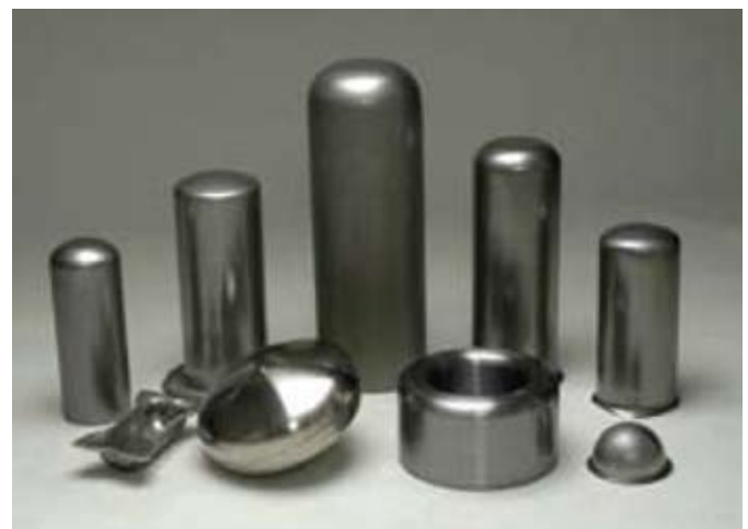
Figure 1 | Parts produced by the deep-drawing of metal. This metal-forming operation uses a press to draw metal so that the depth of the draw is deeper than the diameter of the punch used. [Courtesy of Etna Products Inc.]
