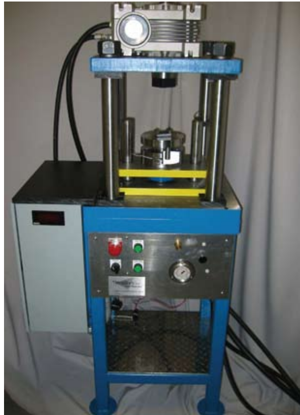
Figure 5 | The Twist Compression Tester is a lab bench test that can evaluate lubricant performance over a range of conditions. The transmitted torque between a rotating annual cylinder and a lubricated flat-sheet specimen is measured. [Courtesy of TribSys LLC]
