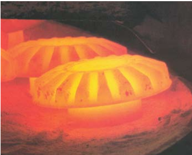
Figure 2 | Hot forging of steel is carried out at temperatures between 1,150 C and 1,290 C. A precision bevel gear placed on a cooling table is shown after undergoing hot forging. [Courtesy of Metalworking Consultant Group LLC]
