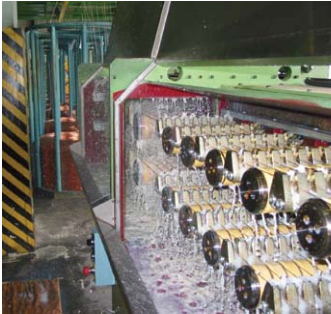
Figure 3 | A high-speed, multi-wire, machine used in copper wire-drawing can reduce the diameter of the wire down to as thin as 44 gauge (0.0020-inches). [Courtesy of RichardsApex Inc.]
